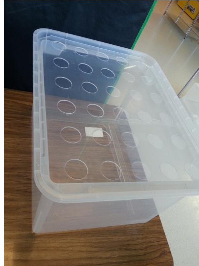
Plexiglass with cut holes to hold the starter plugs and cut to fit in the top of the hydroponic system box
