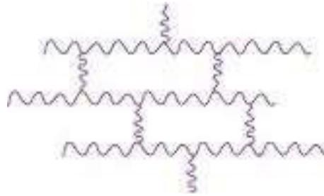
This structure is similar to that of cellulose and collagen. It is also the structure of strengthened rubber. The polymer chains found in natural rubber are very flexible and become fluid like when heated. It was discovered that when sulfur was introduced to natural rubber that the sulfur created links between the long polymer chains in the rubber and significantly improved the response to temperature. Hence the rubber used in tires is a cross-linked polymer.
