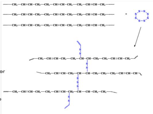
The bonds between the atoms both in the polymer itself as well as the bonds in the shorter cross links have specific strengths. When a material, such as a liquid in the case of this activity, is introduced to the polymer, changes in the polymer can occur if the force of attraction between the fluid and the atoms in the cross link system is stronger than the bonds between the atoms in the cross link polymer system.
