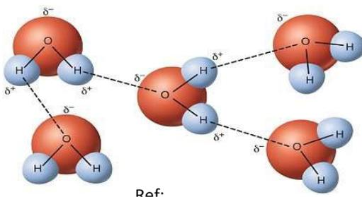
When the water is heated up, thermally induced vibrations are introduced into the water system. At a certain temperature the thermally introduced vibrations will be stronger than the hydrogen bonds between the water molecules and the hydrogen bonds will be broken. More of the water molecules will have more of the charged regions available to interact with the atoms in the polymer.
