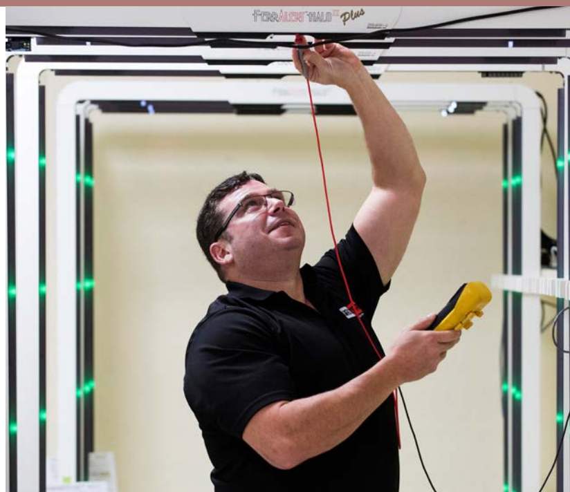
A LASER-TEC graduate tests ferromagnetic detectors used for magnetic resonance imaging safety.
