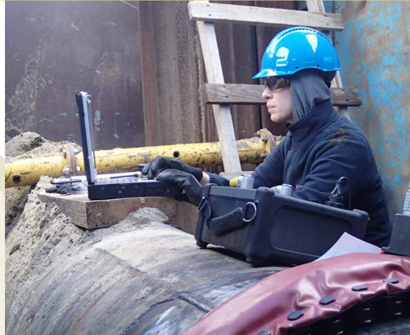
Guided wave testing is one of the ways that welding technicians check buried pipelines for corrosion.
