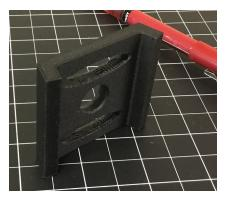
Additionally, now that the part is digitally stored, not only can spare part versions be fabricated in preparation for next year's harvest cycle, but improvements can be made to update the design as needed. And as new 3D printing materials become available, the parts can be further improved upon and allow for low cost preventative maintenance.
