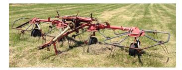
Recently, such a stressful breakdown situation occurred to a regional beef farmer in during the middle of ideal hay harvesting operations. While aerating the cut hay using a hay tedder machine, a bolt came loose and a metal spacer (referred to as a Tedder Tooth Support) component fell off which is used to hold the spinning forks of
