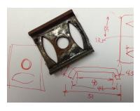
With rain in the near forecast and no replacement spacers available, SCC was able to quickly duplicate the model and fabricate a spacer replacement. The computer model was generated in less than 7
