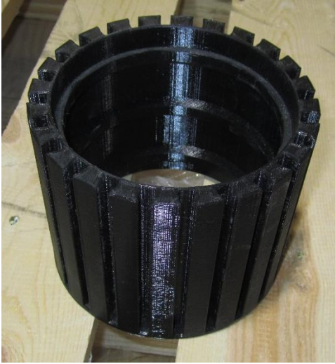
Figures 3 and 4: Final low cost AM produced sanding machine replacement part
