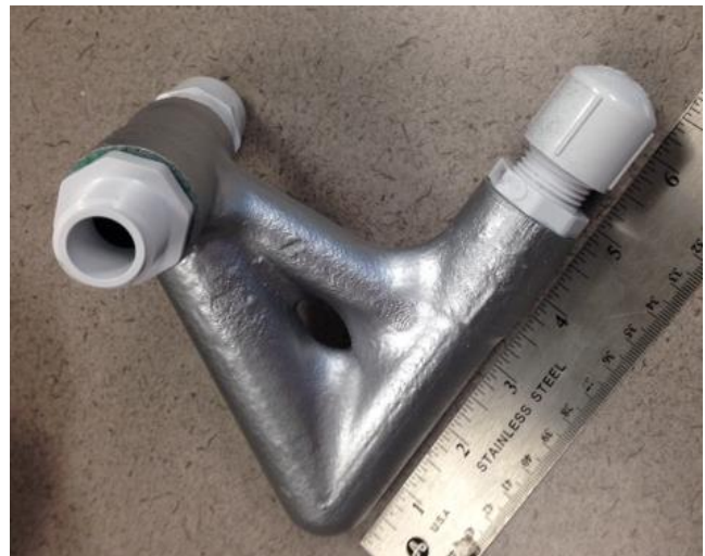
Figure 8: AM produced final part, with silver finish coating
