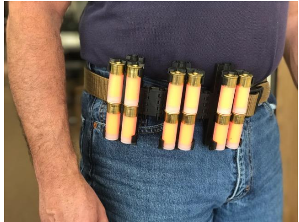
Figure 6: MCE AM product: custom belt shotgun shell holder
