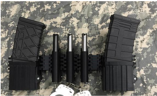
Figure 8: Tactical magazine low cost AM product
