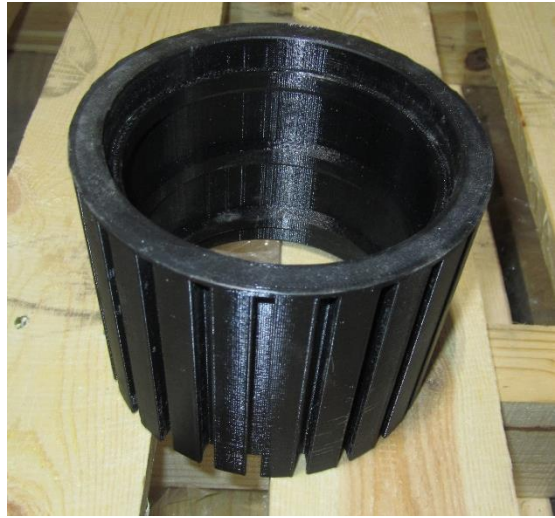
Figures 3 and 4: Final low cost AM produced sanding machine replacement part
