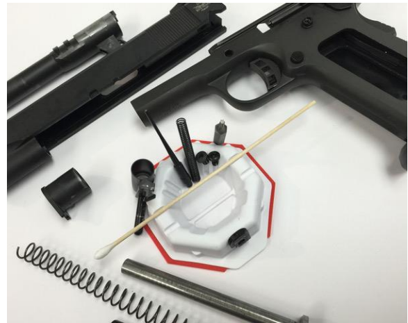
Figure 10: Magnetic tool holder, low cost AM produced internal component
