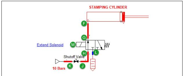
7. What should be the air pressure measured at the port marked with a "G"?
