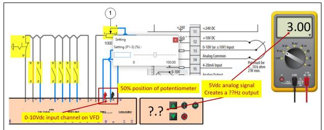
5. What will be the output frequency on this VFD, if 3 Vdc is on the analog input channel?
