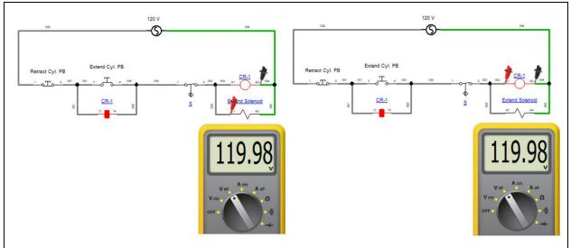
3. The Extend Solenoid is not shifting the pneumatic valve. What could be wrong based on the readings of the two meters?
