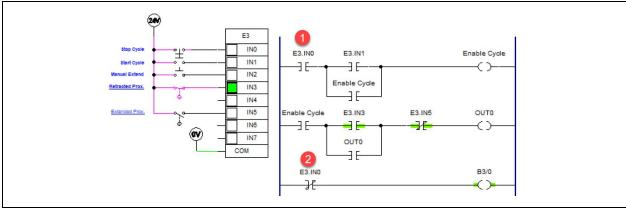
1. With the Stop Cycle push button activated, which one of the contacts marked with a number will have a highlight? (PQ3\_13)
