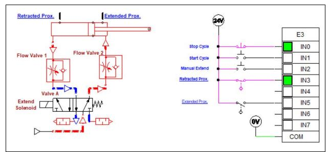
9. Based on the input indicator lights on the PLC input module, what would be the position of the cylinder rod for the pneumatic circuit? (QP4\_9)
