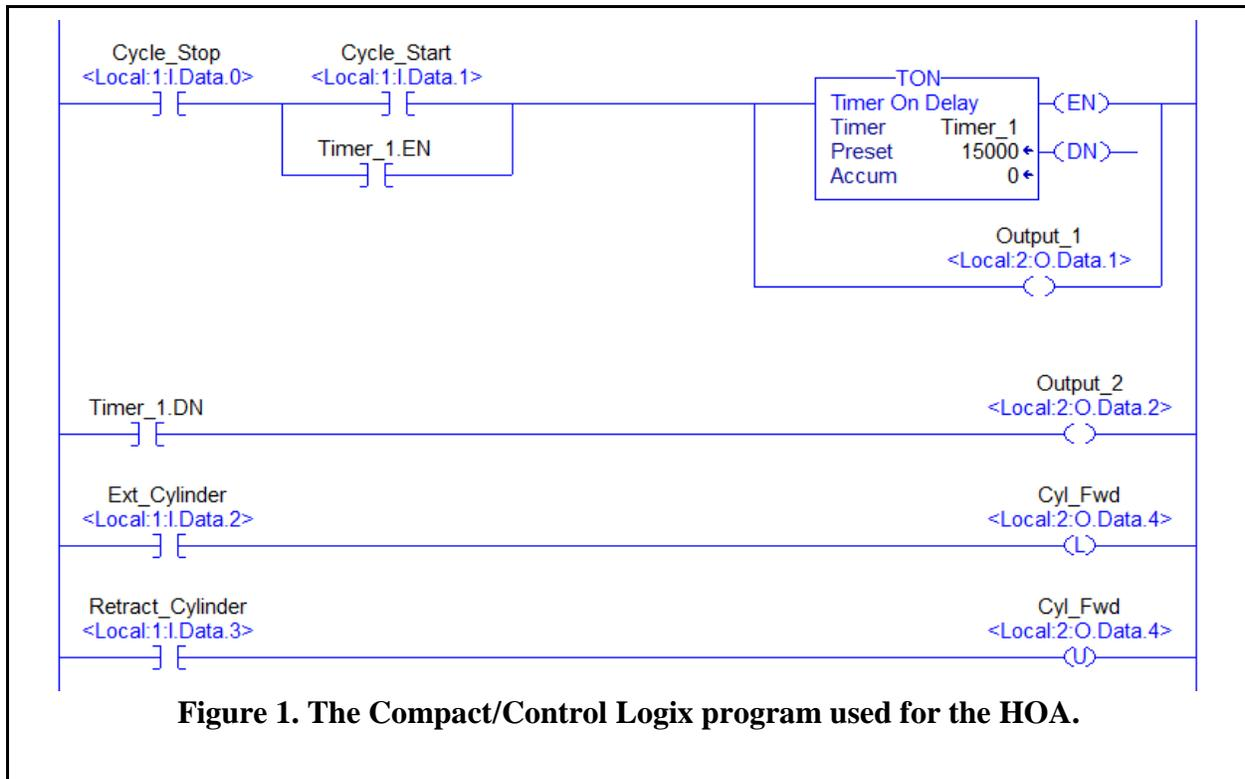
**Figure 1. The Compact/Control Logix program used for the HOA.**
