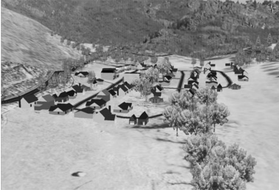
FIGURE 1: A computer-generated 3-D model of a small neighborhood, created using CommunityViz software. The land and trees are real, but the buildings are only proposed. The scene models a meadow high in the mountains. With the software you could “walk” through, explore, alter, and analyze the impact of development proposals.
