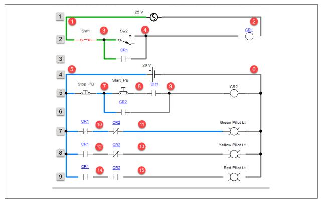
Figure 2. IND220 Lab 2.3 Circuit 1, with line and wire numbers added
