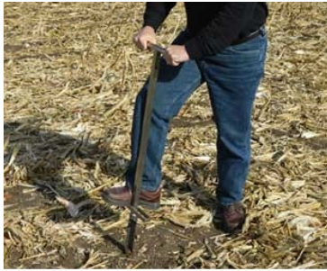
Using a soil probe to collect a soil sample.
