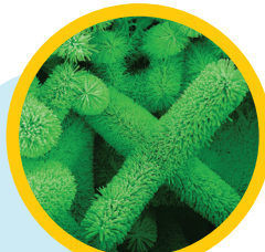
Nanowires Grown for Potential Biosensing Applications. Credit: National Cancer Institute, Z.L. Wang, Ph.D.
