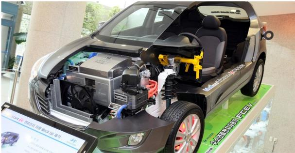
The top image shows a cutaway of the Hyundai ix35 FCEV. The fuel cell stack is located in the front engine compartment, and the hydrogen tanks are positioned behind the rear passenger area. The motor is located at the rear of the vehicle.
