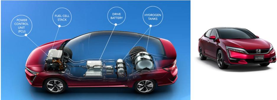
The top-left image is a cutaway diagram of a red Honda Clarity Fuel Cell. It shows the internal components: the Power Control Unit (PCU) at the front, the Fuel Cell Stack in the middle, the Drive Battery located behind the fuel cell stack, and two Hydrogen Tanks at the rear. The top-right image shows the exterior of the red Honda Clarity Fuel Cell sedan.
