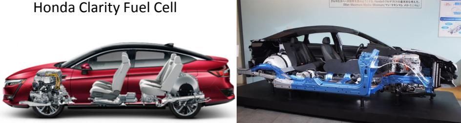
The bottom-left image shows the chassis of the Honda Clarity Fuel Cell with the seats removed. The bottom-right image shows the interior of the car, highlighting the fuel cell stack and battery pack located under the front seats.
