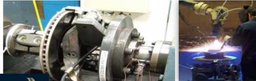
Aluminum brake rotor with thermally sprayed wear resistant coating
