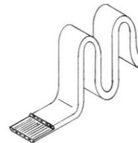
Continuous reinforced thermoplastic material, tape used for woven sheets (thermoforming), filament winding or pultrusion
