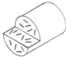
Typical short fiber thermoplastic material, granules with fiber length of approx. 2 to 4 mm, resulting fiber length in a part of approx. 0.4 mm
