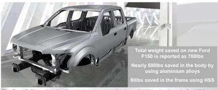
The Ford F150 truck is the first high volume application of LWV technology in the USA Ford worked with aluminium suppliers & technology providers to ensure capacity is in place Further Capacity will be put in place in the USA as further models require LWV technology Shifts the aluminium needle, but still less than 5% of total Auto Body Sheet requirement
