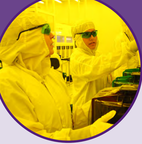
Technicians load 300mm Front Opening Universal Pods (FOUP) onto a tool at SUNY Polytechnic Institute's semiconductor fabrication facility.
