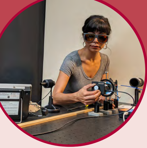
A LASER-TEC student works with a laser beam profiling system.
