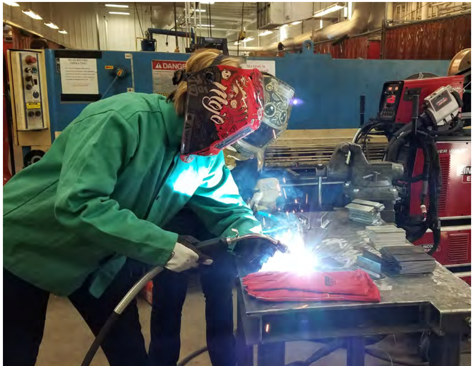
A female welder learns a shielded metal arc welding technique from another woman with industrial welding experience at the Women in Welding Competition.
