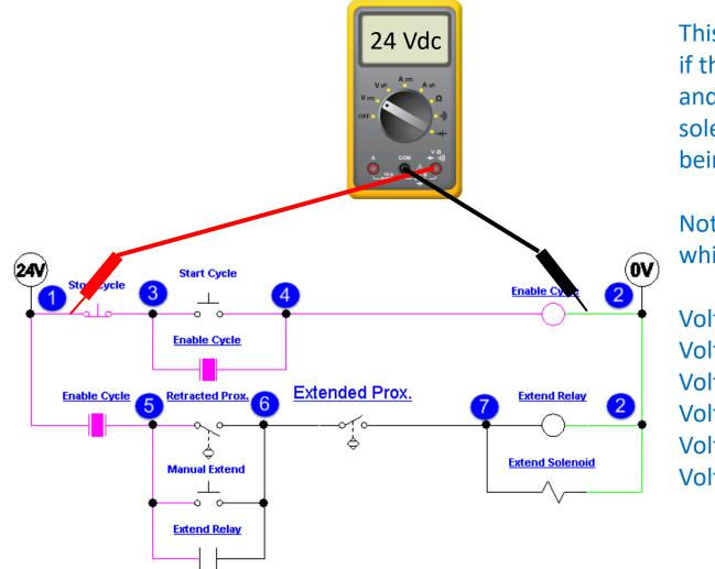
This slide will show the voltages that should be measured if the first rung is energized (Enable Cycle is pulled in), and the second rung does not have the relay and solenoid powered, due to the N.C. Extended Prox switch being actuated (between nodes 6 & 7).
