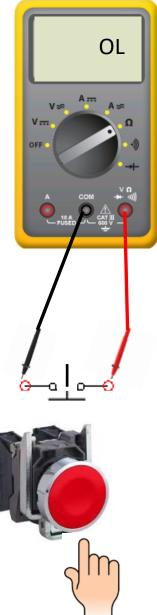
Many times a user must test a Normally-closed pushbutton when it is out of the circuit, to determine if it is faulty.
