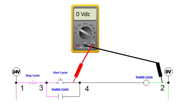
This slide shows that between nodes 4 and 2, there will be no voltage. This is due to the fact that neither the Start Cycle pushbutton, or the Enable Cycle relay are actuated.
