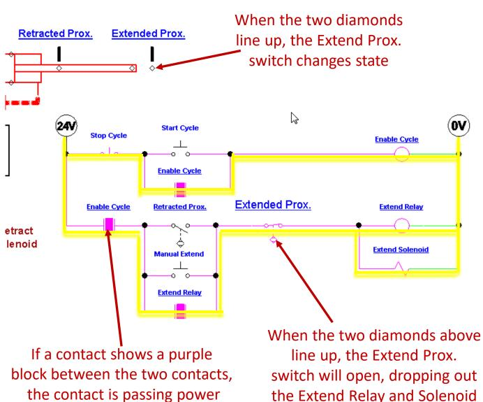
This graphic will give a further in depth explanation of the electrical circuit.
