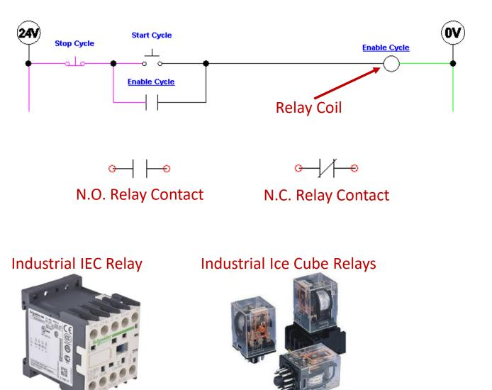
This slide shows a basic the symbols and actual devices for an electro-mechanical relay. A relay is used as a logic device in a ladder logic circuit. The relay typically has Normally Open (N.O.) contacts that has no continuity in it's deactivated state. It also may have Normally Closed (N.C.) contacts that should measure 0 ohms (full continuity) in it's deactivated state.
