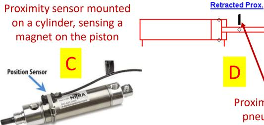
D D Proximity Sensor in a pneumatic circuit
