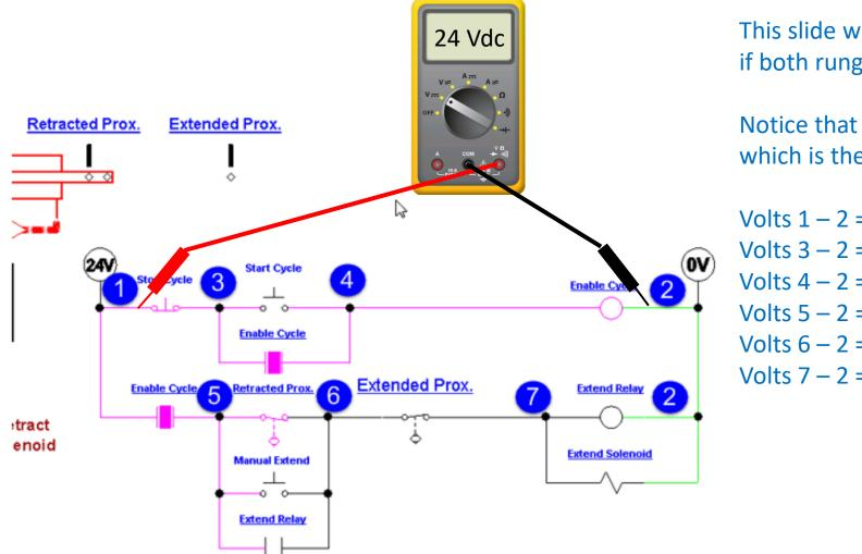
This slide will show the voltages that should be measured if both rungs are powered, and the solenoid is energized.
