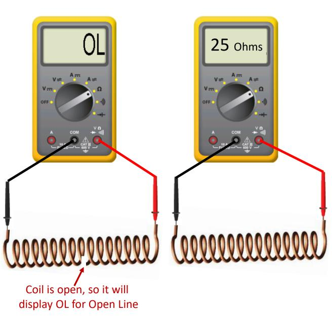
To verify that a solenoid coil is good, the user can measure the resistance when it is not connected in a circuit.
