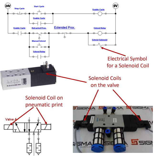
This slide will show the solenoid actuated directional control valve. The graphic in the lower left corner will show a 5/2 valve, that is dual solenoid actuated.
