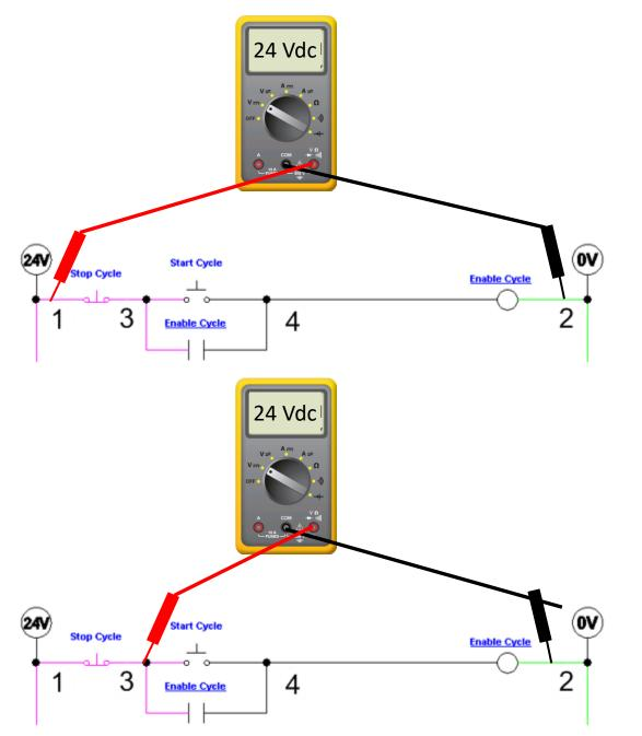
This slide shows what voltage will be measured across the 24Vdc power lines. It is 24Vdc, as shown in the top diagram. Notice that the dial has to be set for DC volts.
