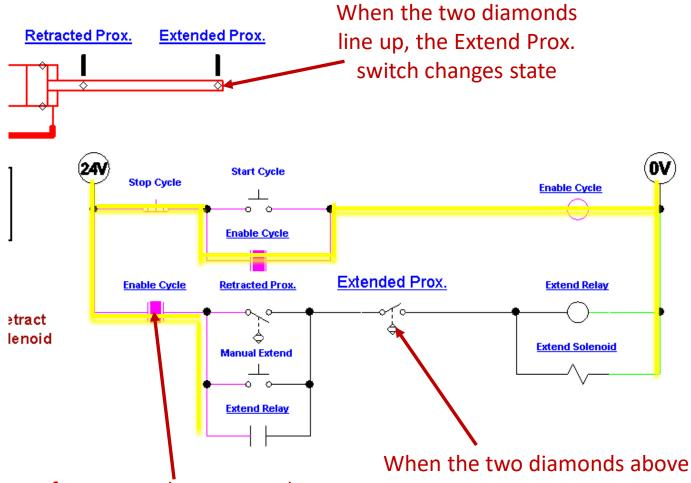
If a contact shows a purple block between the two contacts, the contact is passing power When the two diamonds above line up, the Extend Prox. switch will open, dropping out the Extend Relay and Solenoid
