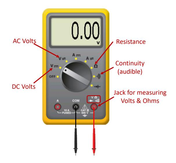
It is important to know how to use a digital multi-meter to perform troubleshooting tasks. This example shows a digital multi-meter that is used in Automation Studio, but is also very similar to any actual digital multi-meter.
