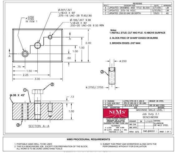
Figure 2. The mechanical print for the Benchwork workpiece.
