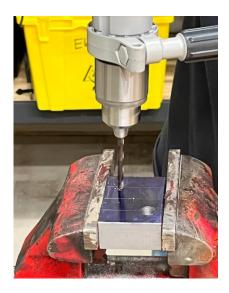
Figure 9. Drilling the holes in the workpiece.
