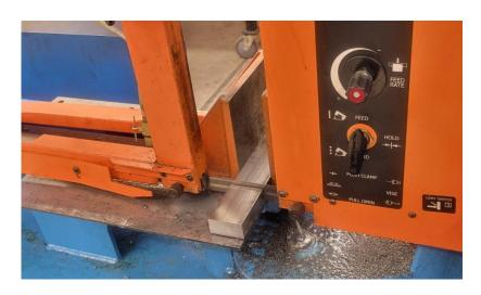
Figure 3. Sawing the block from a piece of stock.
