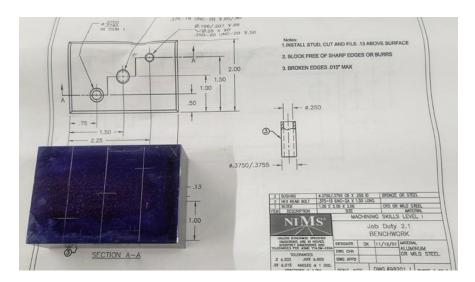
Figure 7. Laying out the hole center points on the workpiece.
