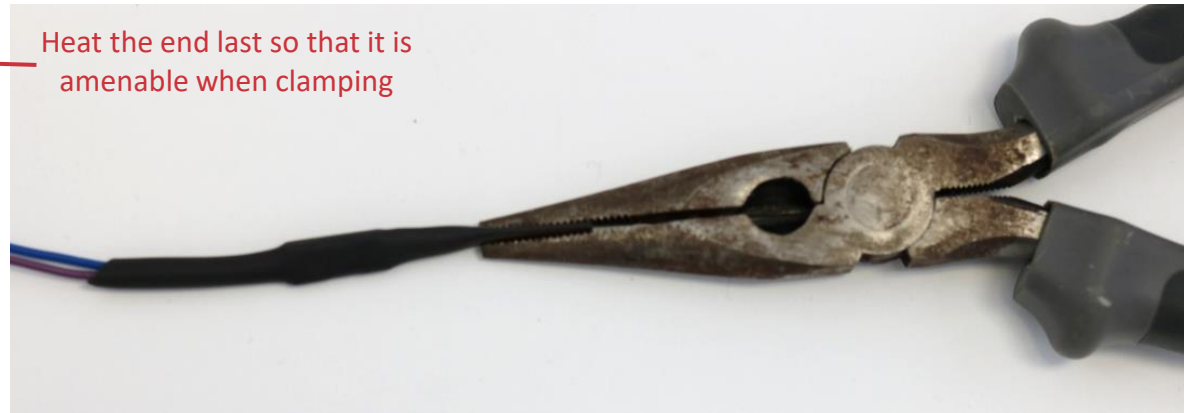
Clamp end of heated material to seal in the thermistor Be sure to not crush the thermistor when clamping material
