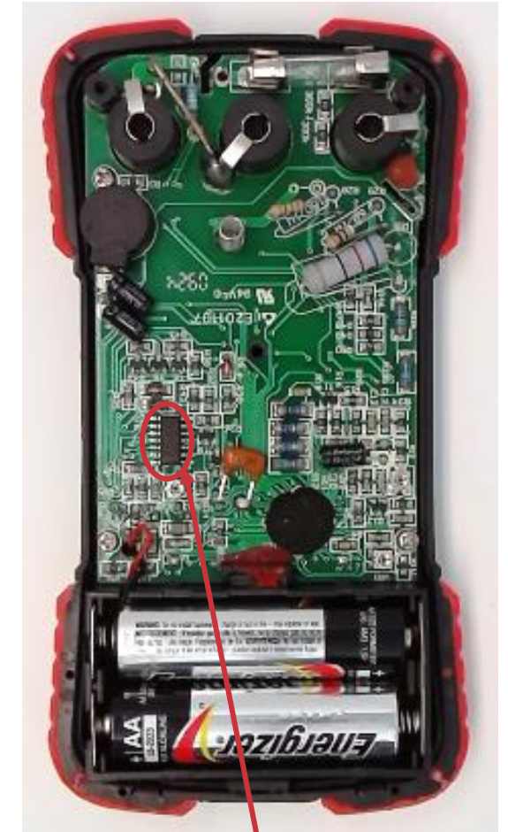
This chip in your multimeter contains multiple transistors
