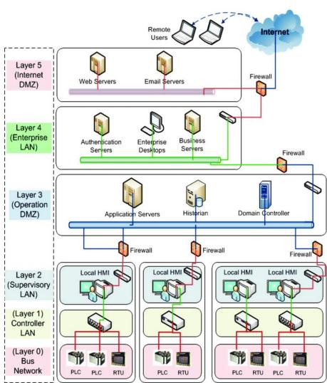
**Examples of SCADA Architecture in RE**
