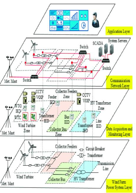
Source: Communication Architecture for Grid Integration of Cyber Physical Wind Energy Systems - Scientific Figure on ResearchGate. Available from: https://www.researchgate.net/figure/Proposed-architecture-of-the-cyber-physical-wind-energysystem-SCADA-supervisory fig6 320312821
