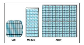
Tiny electrical contacts enable the electric current to run through each PV cell. Somewhat larger contacts are attached to the side of each PV cell. Many PV cells are then connected together to form a solar panel, or module. Each module has a junction box on the back with wires available to connect one module to another. Modules can be connected to an array of almost any size to meet a range of electrical demands.
