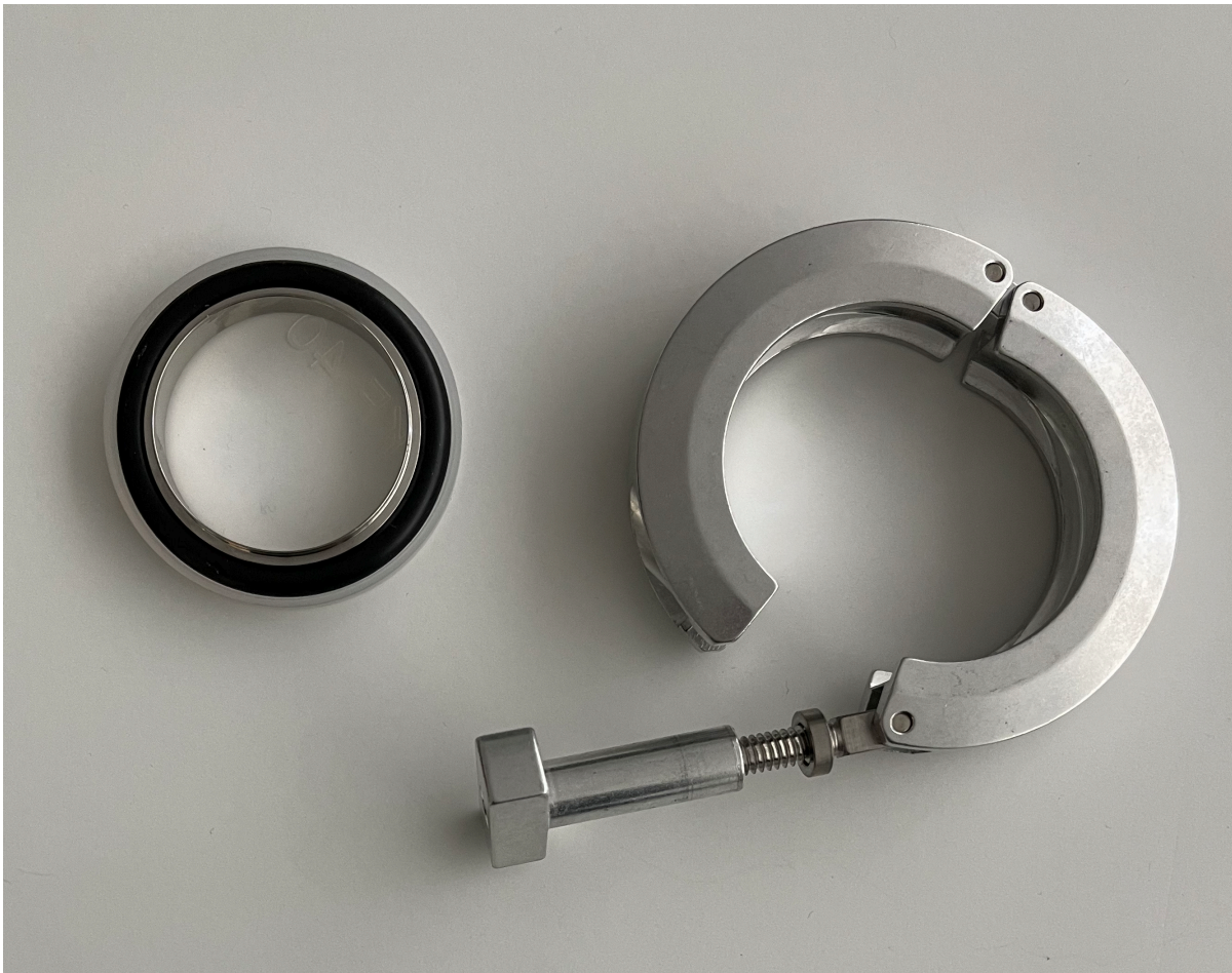
Figure 3.6. KF fitting, centering ring with elastomer O-ring (left), and clamp (right). Photo provided by Elena Brewer, SUNY Erie Community College.
