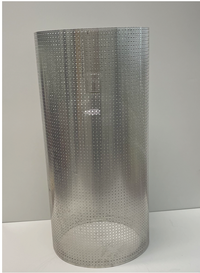
Figure 3.18. A Pyrex bell jar chamber from Figure 3.17 covered by the metal protective shield/guard. Photo provided by Richard Hill, SUNY Erie Community College.
