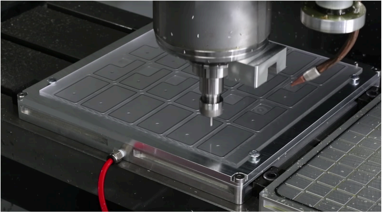
Figure 1.6. A work piece is held in place with vacuum chucks while it is being milled. Source: Pierson Workholding website, https://piersonworkholding.com/media/.
