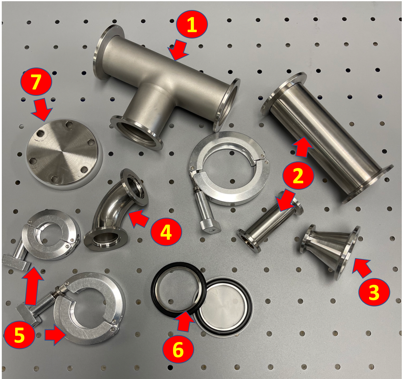
Figure 3.12. Vacuum flange fittings: 1 – tee, 2 – nipple, 3 – reducer, 4 – elbow, 5 – KF clamp, 6 – centering ring with fitted O-ring, 7 – CF pipe end fitting. Photo provided by Elena Brewer, SUNY Erie Community College.
