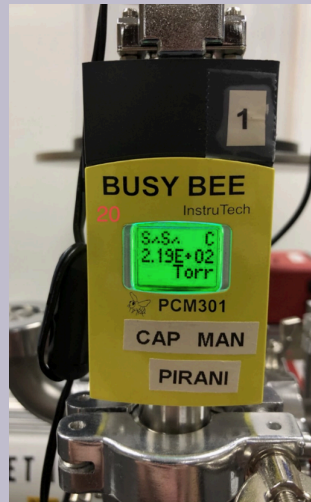
Figure 4.14.c. Capacitance manometer / Pirani gauge measurement. Photo provided by Nancy Louwagie, Normandale Community College. Photo edited by Gigi Bocek.
