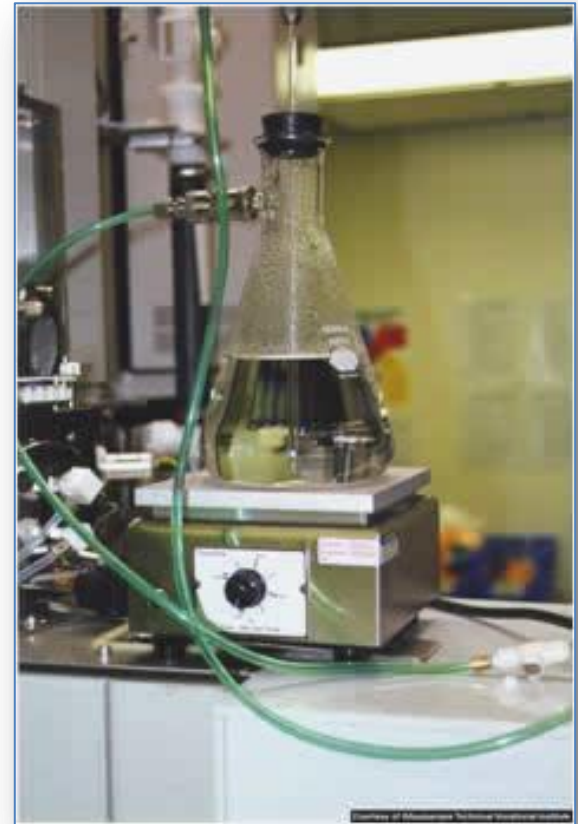
Bubbler used to generate steam for wet oxidation process
