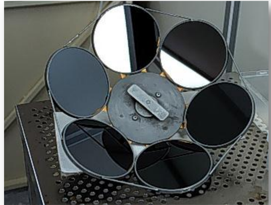
Single planetary for Evaporator. Evaporator can hold several planetary units.
