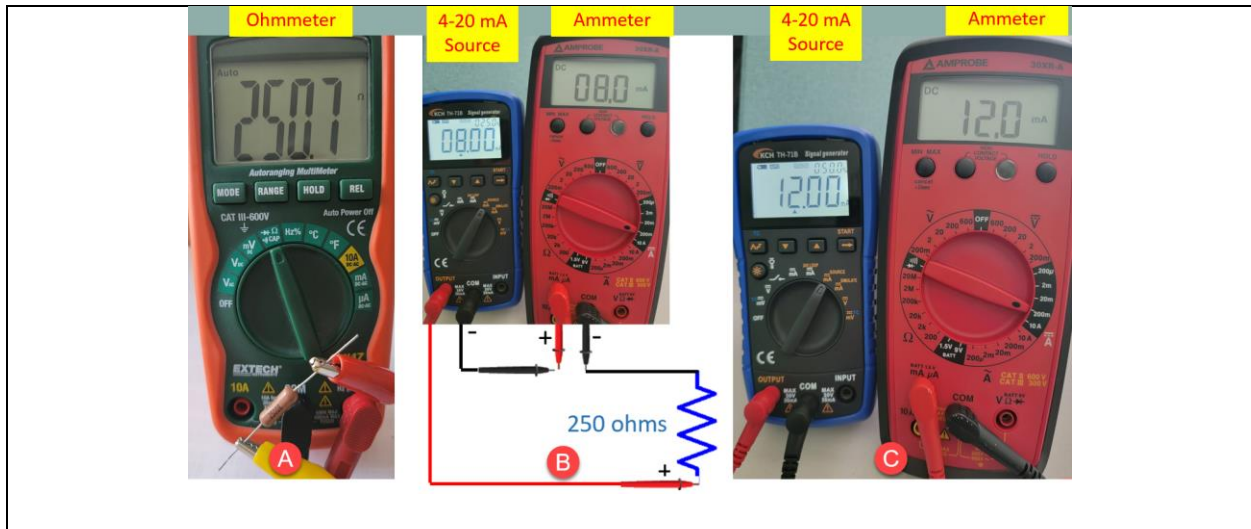
Figure 2. Sourcing and Measuring Current.
