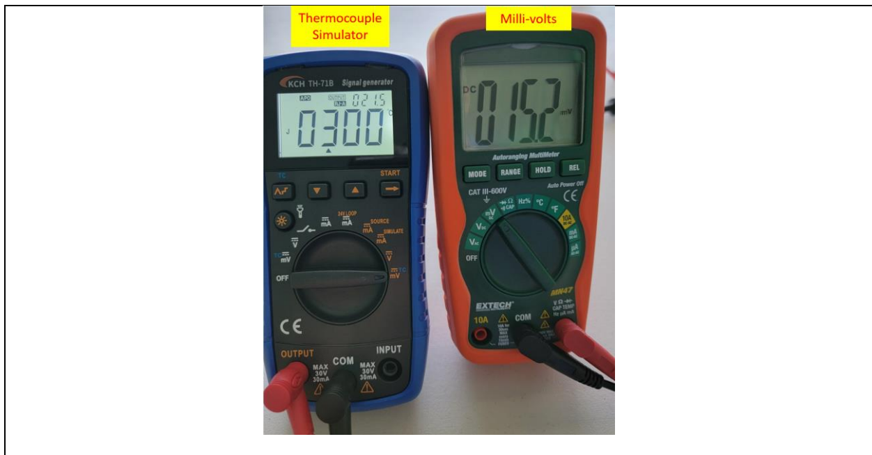
Figure 4. Signal Generator simulating a Thermocouple.
