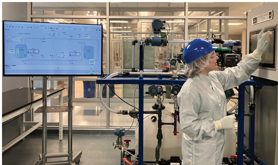
Biotechnology students learn how to operate distributed control systems such as DeltaV.
