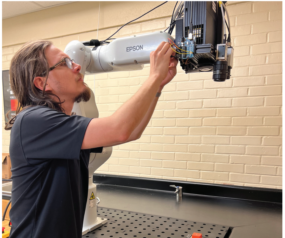
A guided particle systems technician, who is a Pensacola State College graduate, installs a new control board to a NAVI end effector.
