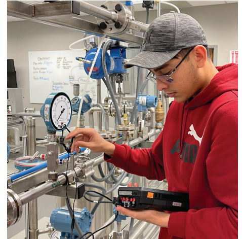
A mechatronics student configures sensors in a pressure gauge using a device communicator in an instrumentation lab.
