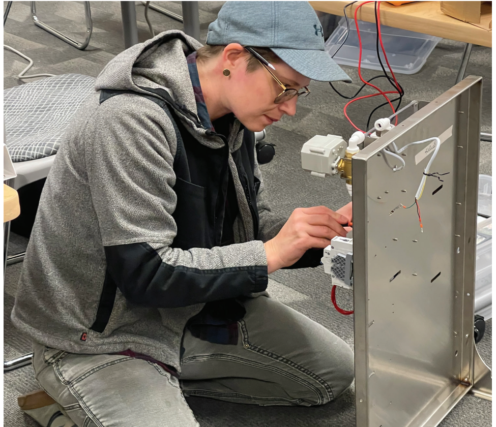
An educator builds a mechatronics instrumentation trainer during a professional development workshop.
