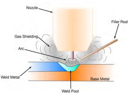
Diagram of the process of non consumable electrode welding
