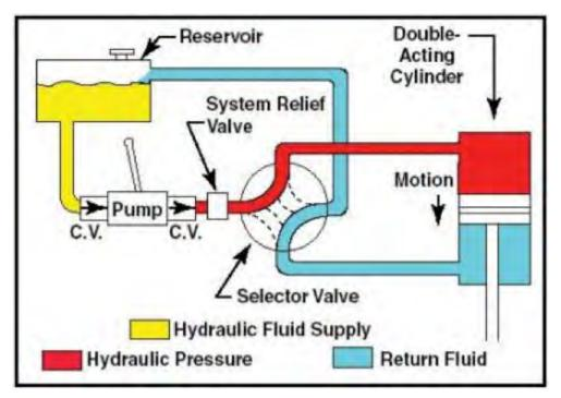
Cutaway drawing showing the internal motion of the piston and how it is controlled
