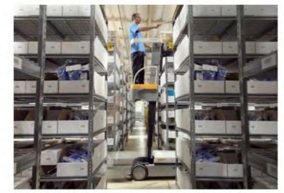
Operation of a high lift used for hand picking.
