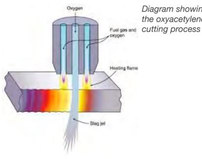
Diagram showing the oxyacetylene
