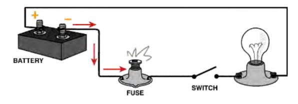
Open circuit with the switch open
