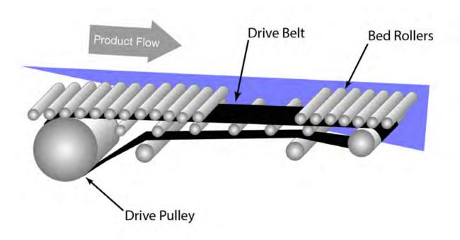
**Movie 5.3** Belt Driven Roller NBC Accumulation Conveyor
