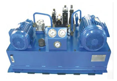
Self contained hydraulic pump assembly with reservoir that is used to power a single piece of machinery or a small area of the distribution center
