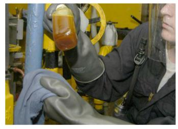
Observing an oil sample for contamination
