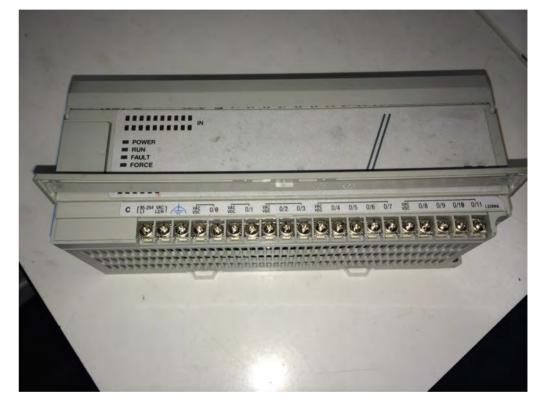
MicroLogix controller showing terminal connections for the outputs
