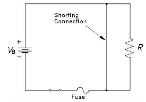
Diagram showing a short circuit
