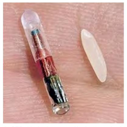
An RFID chip that is compared in size to a grain of rice. The chip is embedded into a label and then attached to a product for identification.
