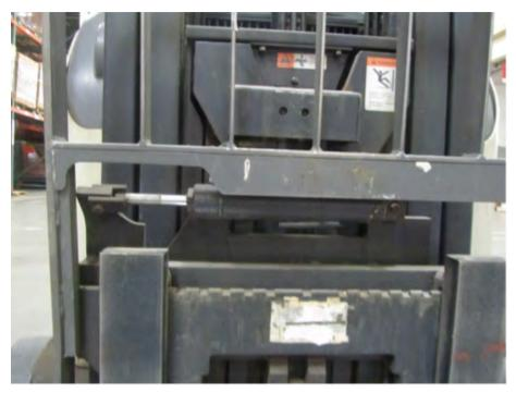
Hydraulic piston for fork movement on a lift truck
