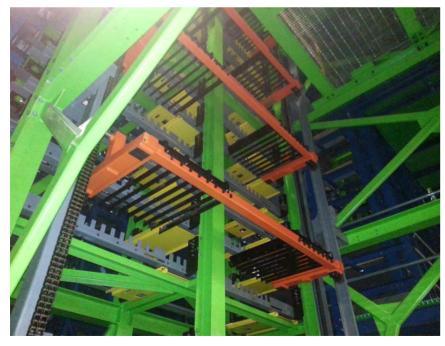
Inside a VRC for raising cartons to different rack levels
