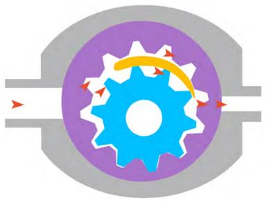
Tap to view a demonstration of a gear pump with internal teeth.
