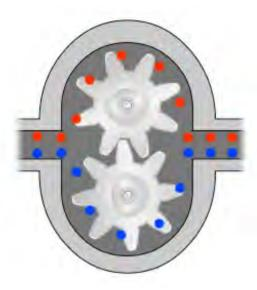
Tap to view demonstration of gear pump with external teeth. Note the rotational direction of the gears.
