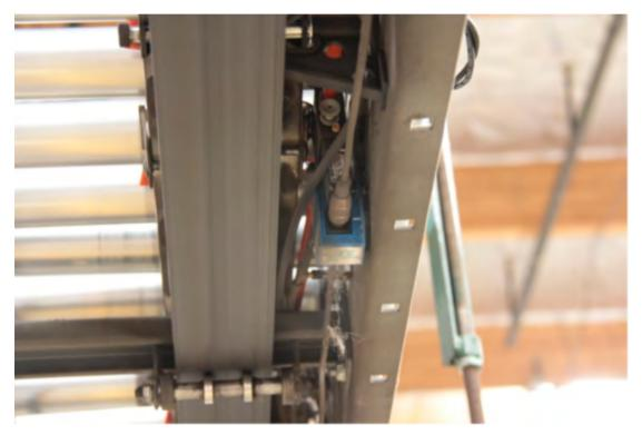
Solenoid actuators converting electrical signals into air pressure control
