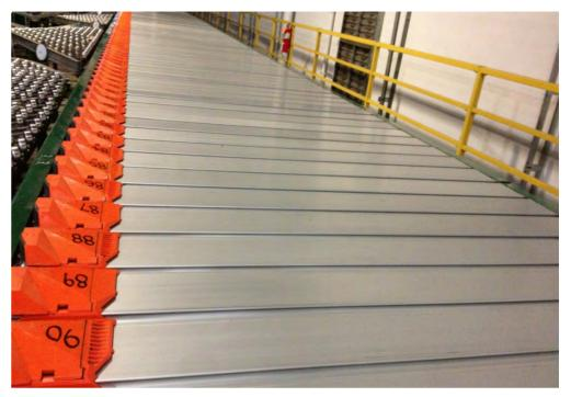
RS200 Sorter PLC controlled conveyor transporting product and sorting by movement of the conveyor shoes
