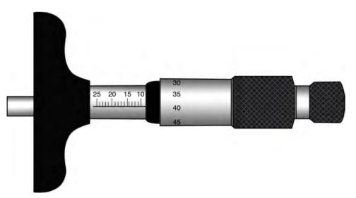
turning the thimble until the measuring points are snug on the device and reading the barrel increments to determine size. The numbered lines represent 100 thousandths (.100), the increments between represent 25 thousandths (.025) and the individual numbers on the thimble represent one thousandth (.001). The exposed markings are added to determine the total.
