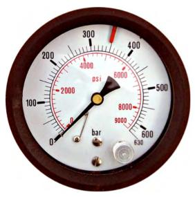
Pressure gauge indicated in PSI and metric systems (bar)
