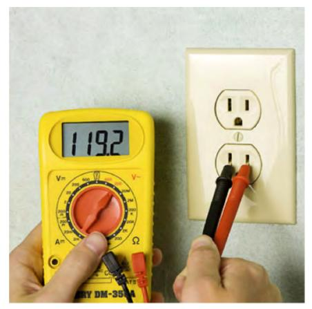
Testing for voltage
