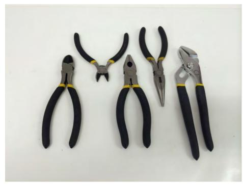
Assorted pliers to apply griping and cutting force to a project
