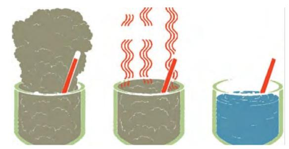
Heat is given off when converting a gas to a liquid, but the temperature can be the same.
