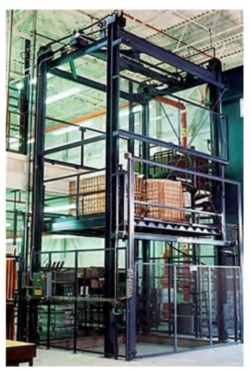
A VRC moving pallets between floor and mezzanine
