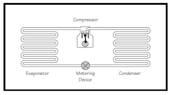
Air Conditioning schematic of the four major parts of the refrigeration cycle
