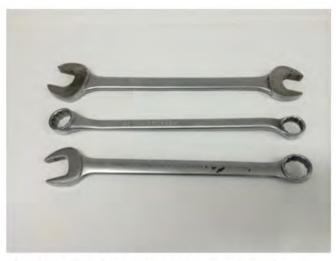
Assorted wrenches and sockets used for applying twisting force to fasteners.
