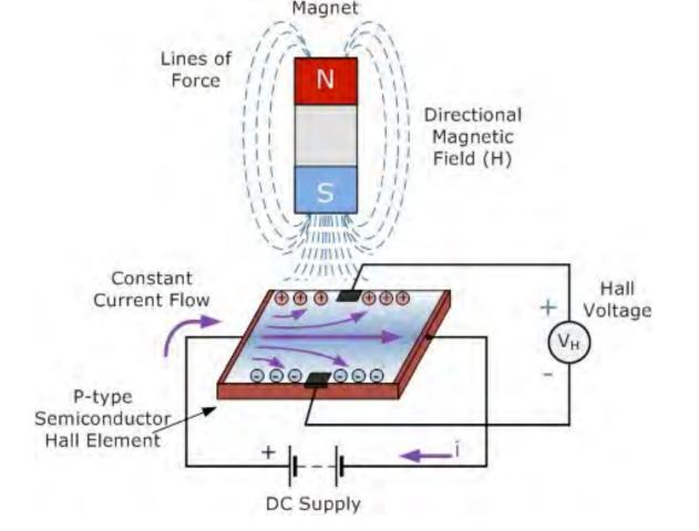
Diagram of the theory of a Hall Effect sensor. Magnetism allows a small voltage to flow through the plate.
