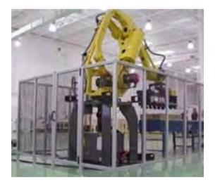
Robot safety cell with fencing
