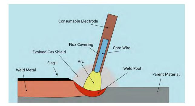
Diagram of the arc welding process
