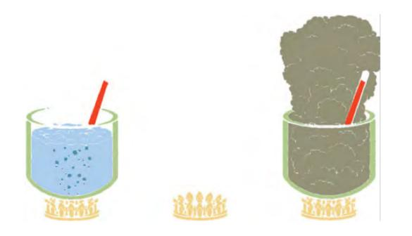
Heat is absorbed to change the state from a liquid to a gas, but the temperature is the same.
