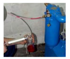
Drawing an oil analysis sample for testing purposes
