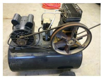
Small sprocket driving a large sprocket to decrease speed and increase torque
