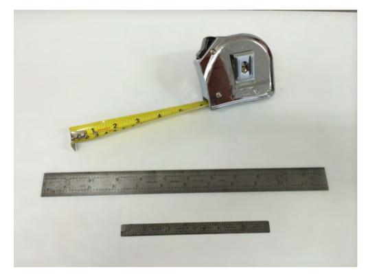
Tape measure and steel rules used for measuring
