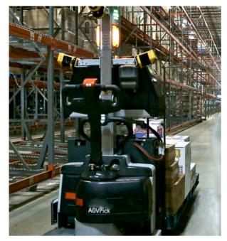
A pallet truck AGV used for product picking
