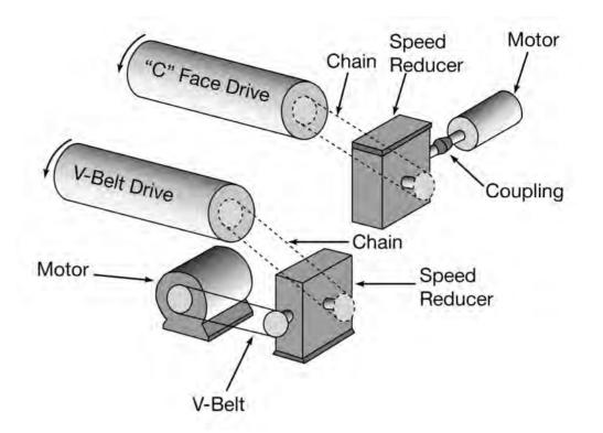
Schematic of two different ways motors and drives can connect to a drive pulley
