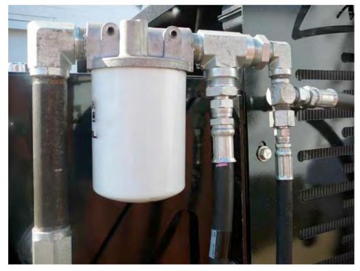
Hydraulic fluid filter to remove impurities from the system
