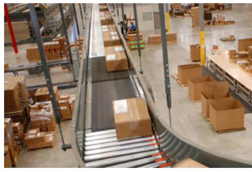
Tap to read about brake meter belts used for carton gapping.
