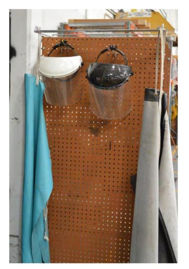
Personal protection equipment used for battery service on lift trucks in a distribution center
