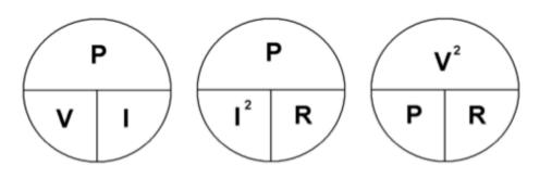
Power equation pie used to determine the amount of work that is being done and to help design a circuit so overloading doesn't occur
