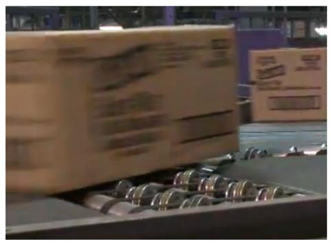
A pop-up wheel sorter with raised wheel section to turn the direction of box travel
