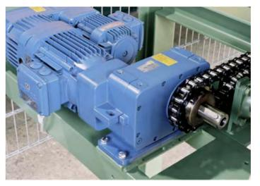
Roller chain being driven by a gear box reduced drive motor
