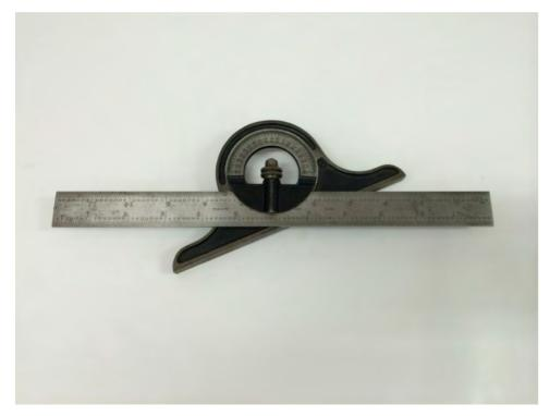
Protractor for measuring angles.
