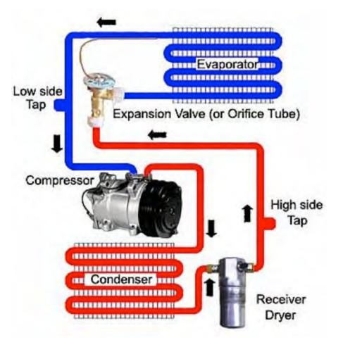
Typical air conditioning system showing the components
