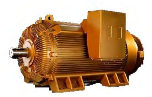
Drive motor with a speed control box and start-up capacitor attached in the square box
