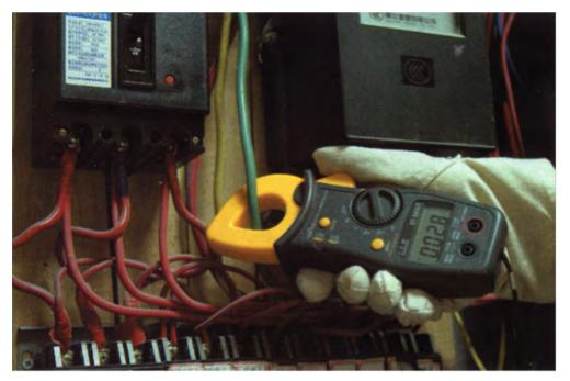
Using a current probe to test current draw
