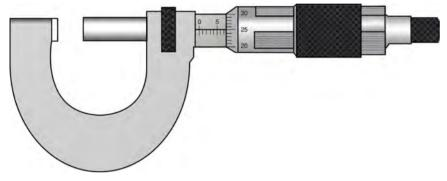
Outside micrometer used for precision measurement.
