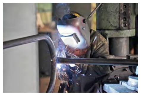
Welder joining round tube
