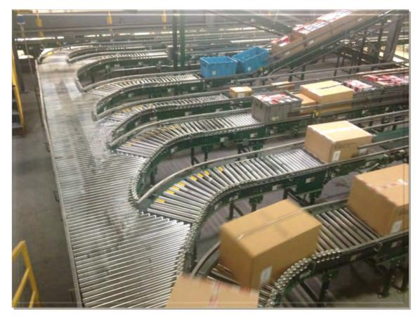
Merge of several conveyors moving product through timed intervals controlled automatically by the PLC controller and/or manually at the operators' control station
