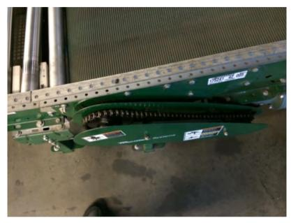
Chain driven rollers for heavy-duty applications
