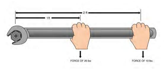
A wrench being used to multiply torque
