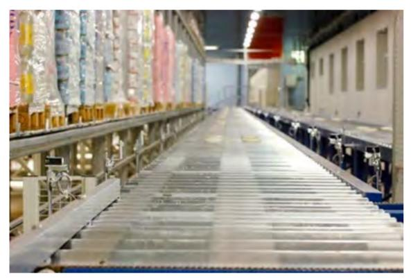
Observe the sensors on each side of the conveyor system. The sensor could count, position or determine the speed of moving products.
