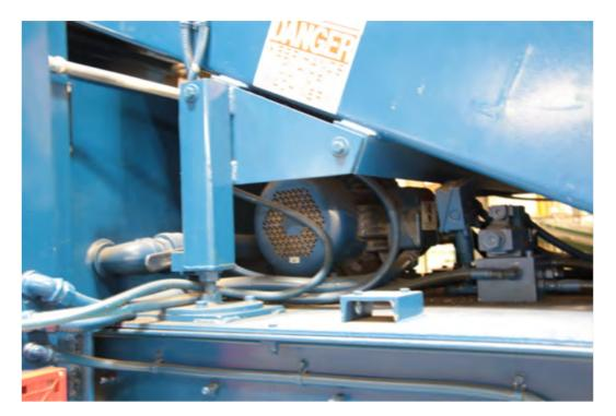
Electric motor powering a hydraulic pump
