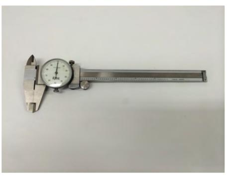
Dial Calipers used for inside, outside and depth precision measurement.
