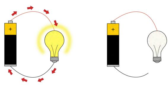
Diagram showing a closed or open circuit
