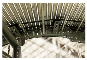
V-belt application for driving multiple rollers on a conveyor system
