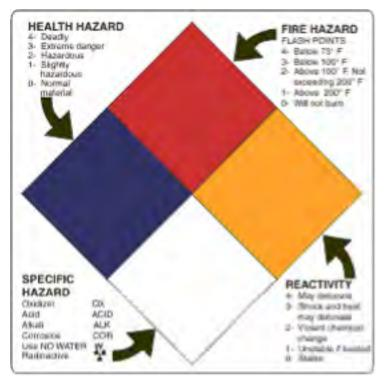
Hazardous Material Identification System poster identifies the type of hazardous material so appropriate precautions can be taken. All materials must be identified. <u>www.nfpa.org</u>
