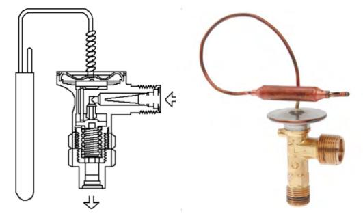
Schematic and Pictorial view of an expansion valve
