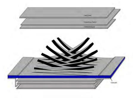
Schematic of vulcanized belt splicing
