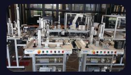
Equipment: MAP 200-205 Robotic Trainers w/Touchscreen HMI, Fanuc Robotic Arm, six-cell automated warehouse storage, FMS 200 SCADA system.
