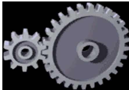
Two meshing gears transmitting rotational motion. Note that the smaller gear is rotating faster. Although the larger gear is rotating less quickly, its torque is proportionally greater.
