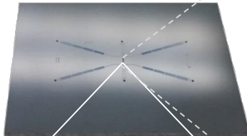
nanoDLD chip mounted in flow cell for fluorescence imaging
