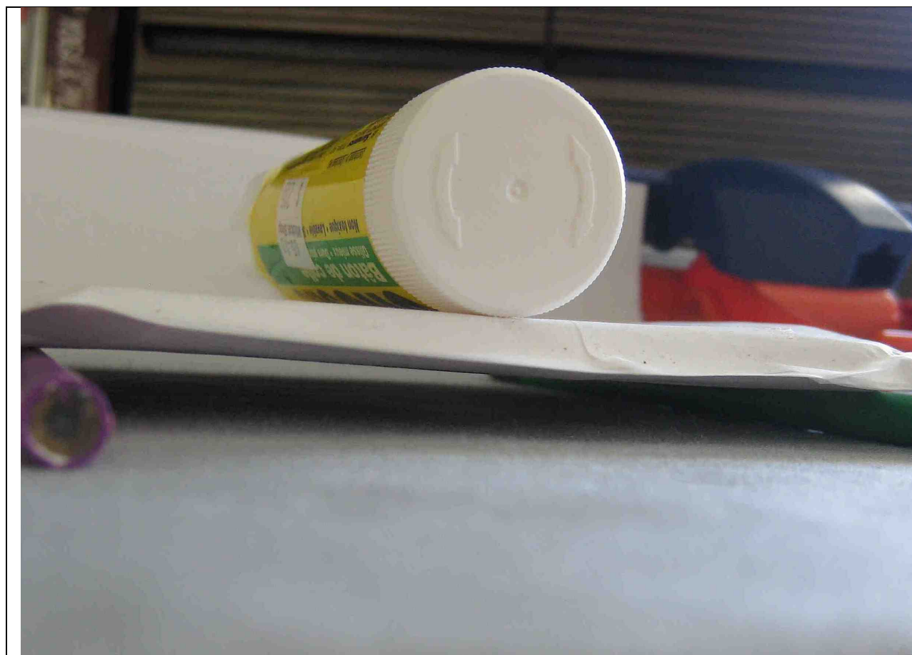
Figure 5: A sandwich panel in 3-point bend supporting a glue stick weighing 60 grams.
