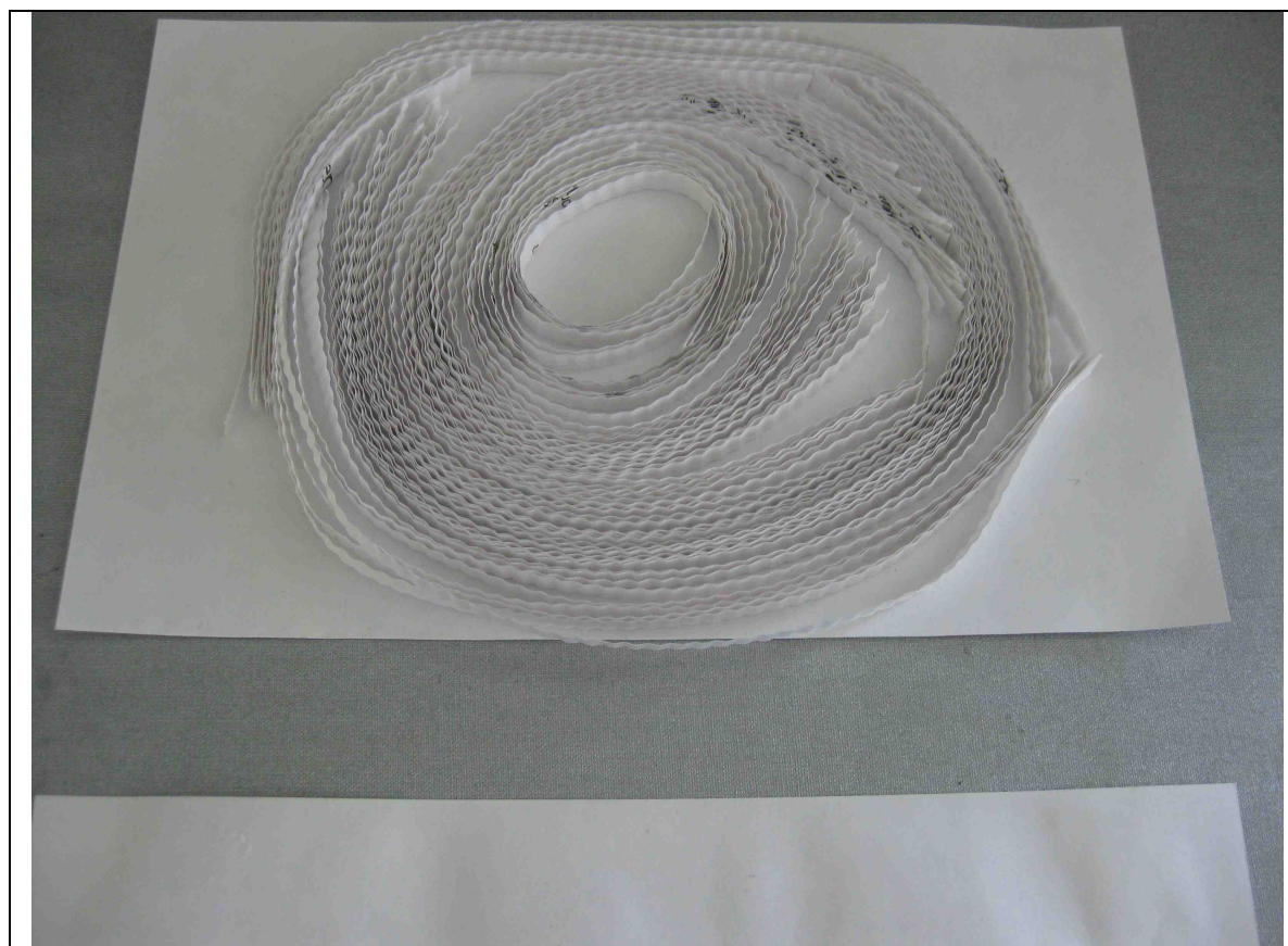
Figure 2: Crimped paper strips are oriented in a spiral and glued to a panel surface sheet.
