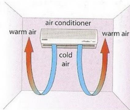
Figure 9.15 Convection currents in an air-conditioned room
