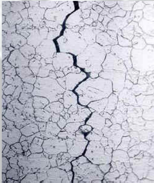
Corrosion for Inconel Following the grain boundaries
