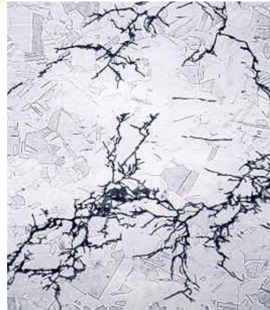
Corrosion for 316 stainless steel
