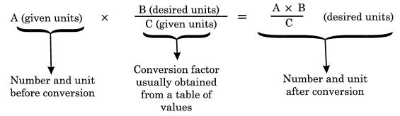
Fig. 1 Unit-conversion process
