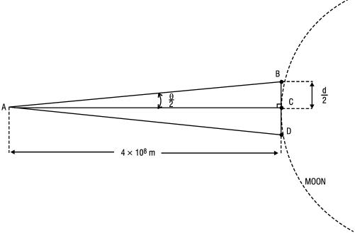
Point A is the origin of the laser on the earth. Segment BD is the diameter of the laser spot when it strikes the moon.
