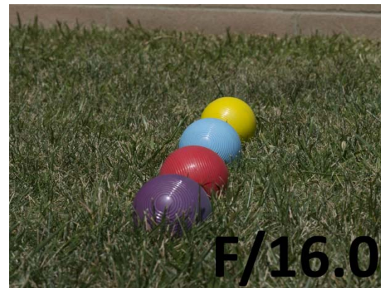
Figure 1-9 The principal of depth of field (DOF) is illustrated by these four images. When the camera's aperture is stopped down (reduced in diameter), the value of the F/# increases and the DOF increases. The grooves in the blue ball are evident in the image shot at F/2.0, but the other balls' grooves are out of focus. When the aperture is stopped down to F/5.0, the red ball's grooves become apparent. Further stopping down the aperture to F/9.0 makes the red grooves sharply focused and shows some detail in the purple ball's grooves, but only at F/16.0 are all balls in focus. The DOF dependence on the F/# is also seen by observing fact that a deeper patch of grass is in focus for higher f-numbers.
