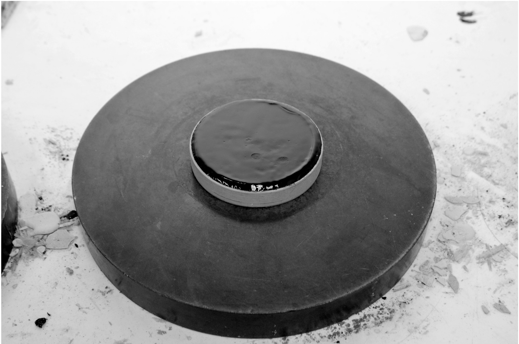
Figure 1-10 Optics blocked in pitch
