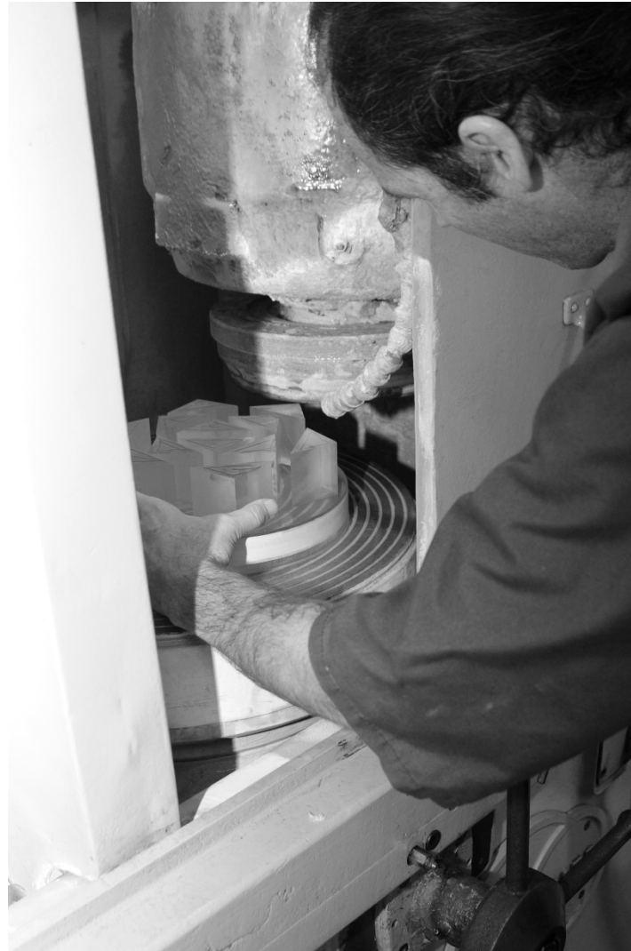
Figure 1-4 Setup of a parallel machining operation
