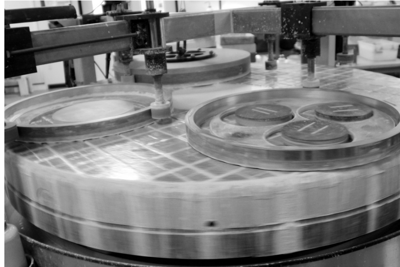
Figure 1-7 Upper left: Hand grinding a block of prisms Upper right: Precision hand grinding an individual prism Bottom: Continuous polishing machine that is pitch-polishing various substrates
