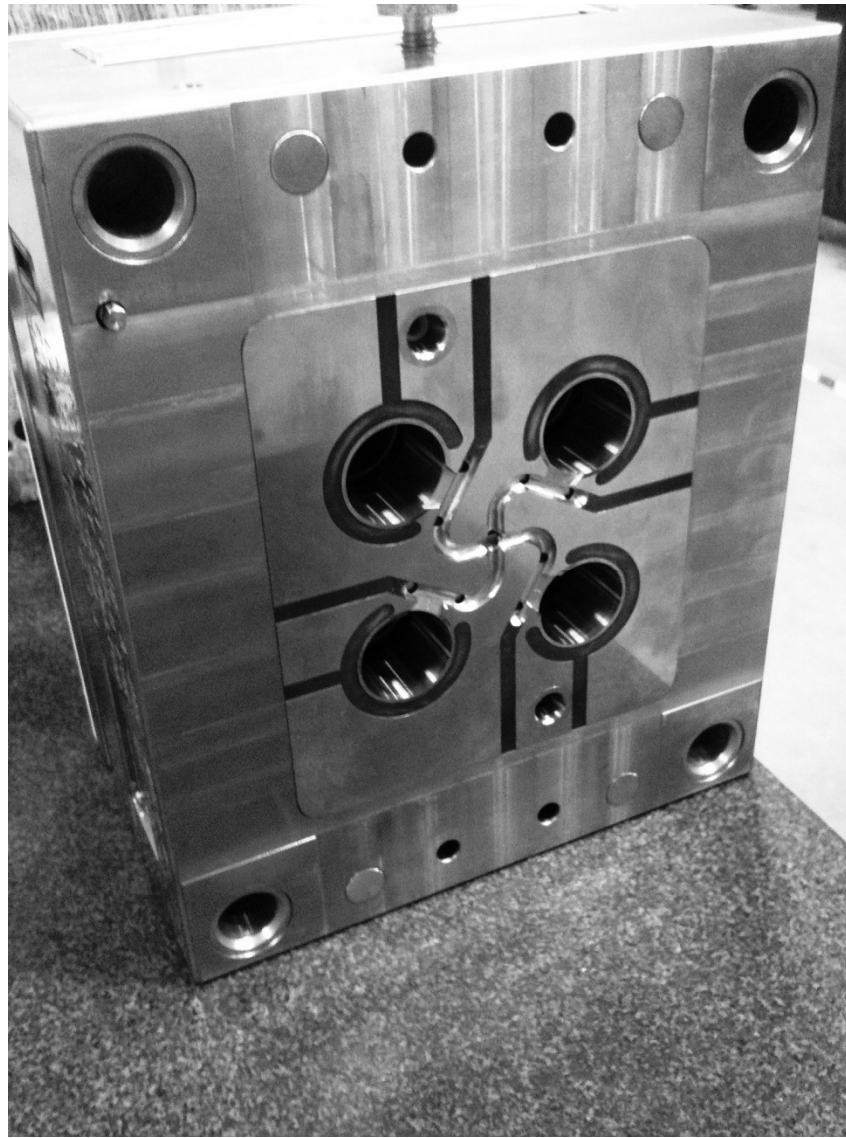
Figure 1-15 Optical plastic injection mold
