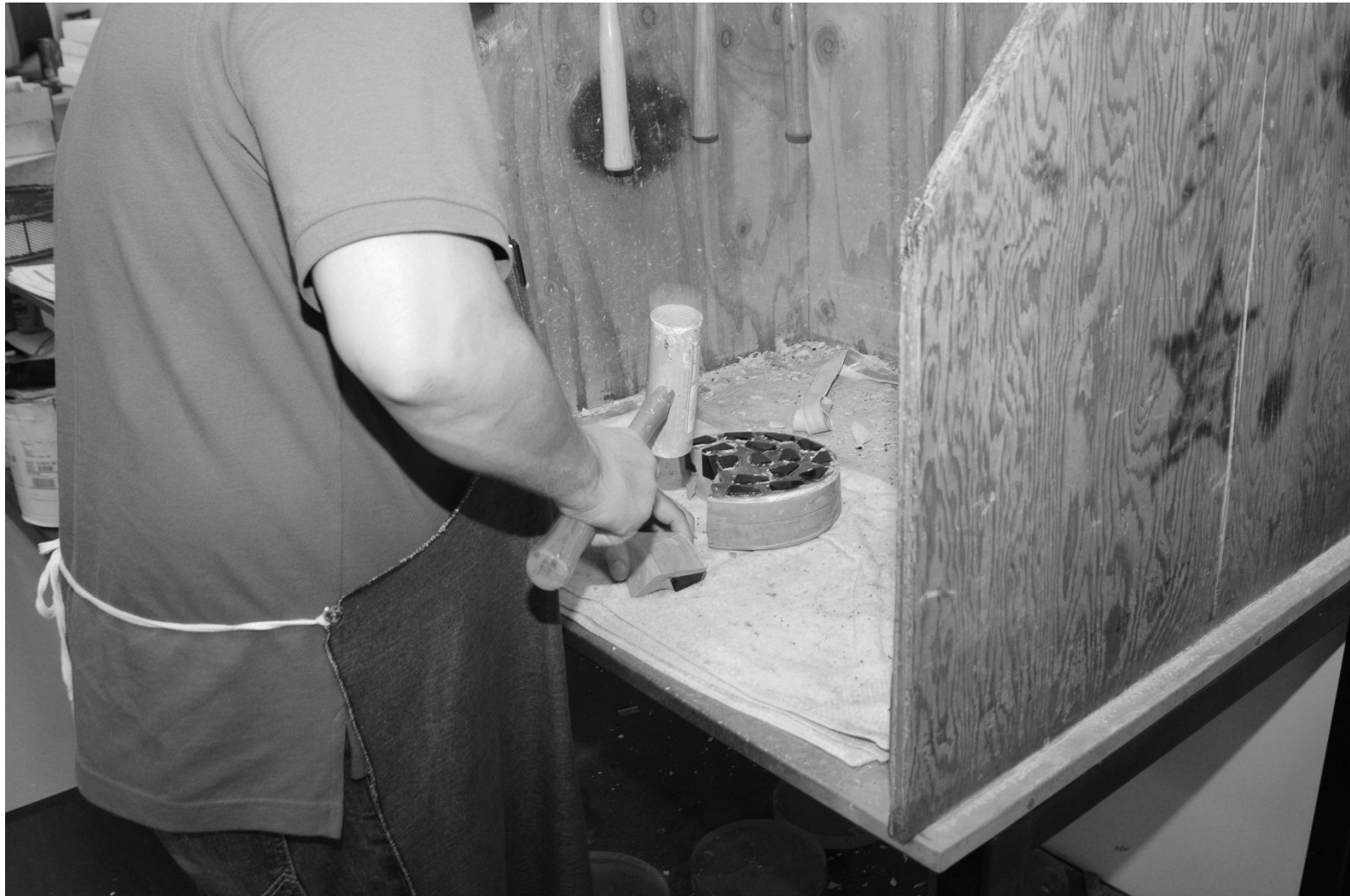
Figure 1-12 Deblocking a plaster block
