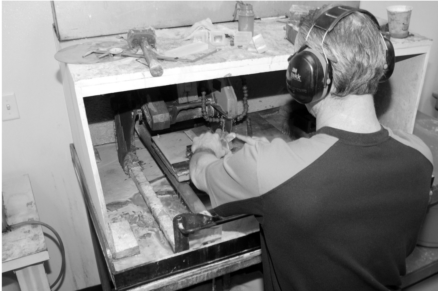
Figure 1-2 Circular saw for intermediate precision cutting
