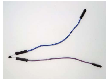
Attach wire extensions to each leg
