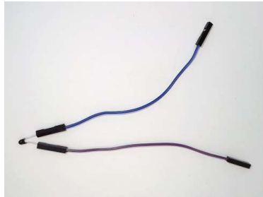
Attach wire extensions to each leg
