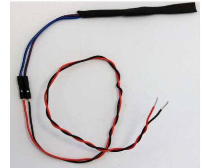
Strip wires jumper wires and connect them to wire extensions
