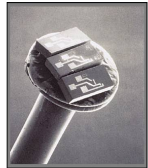
Three MEMS blood pressure sensors on a pin head [Photo courtesy of Lucas NovaSensor, Fremont, CA]
