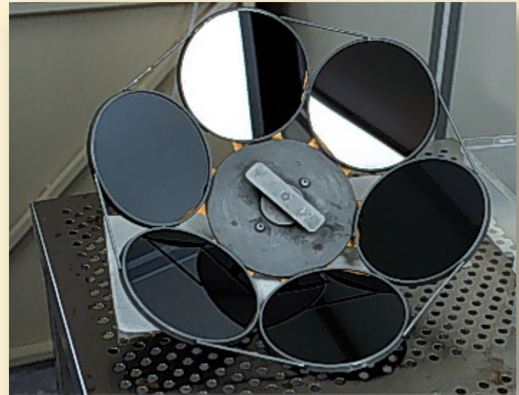
Single planetary for Evaporator. Evaporator can hold several planetary units.
