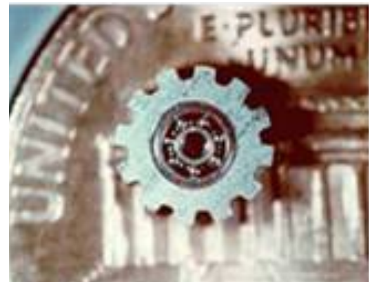
This LIGA micromachined gear is used for a mini electromagnetic motor [Image courtesy of Sandia National Laboratories]
