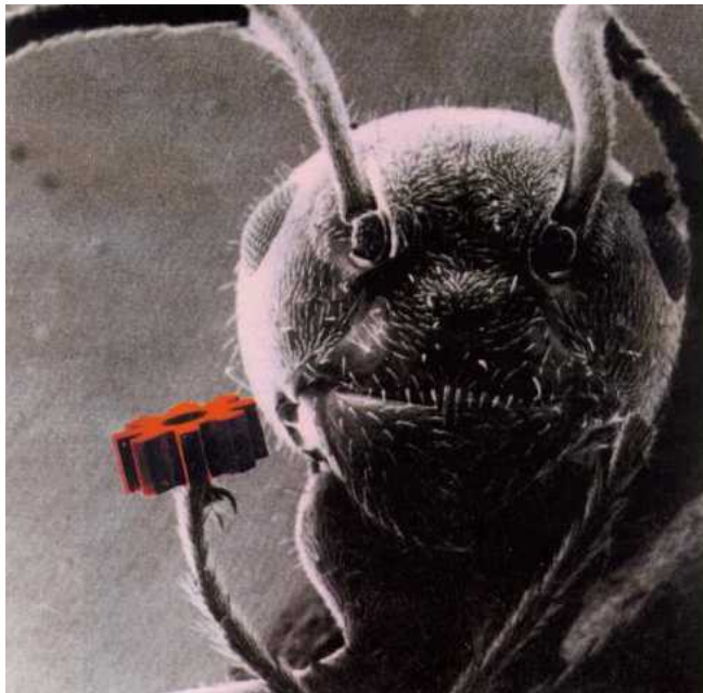
Ant with a LIGA micro-gear. [Image courtesy of Rorschungzentrum Karlsruhe, Germany]
