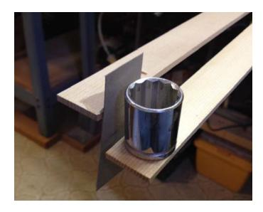
Aside: Wood displays a property known as creep. That means that it continues to deform slowly after a load is applied. The beams used in this experiment may creep when loaded, so you may notice that your test beam continues to move just a little. Rather than try to wait until it stops creeping, record the deformation right after applying the load.
