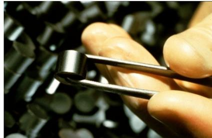
Uranium fuel pellet made from compaction of Uranium Dioxide powder. Not in enriched form here.
