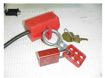
The function of the item is to enclose the plug on an electrical device's cord, and to allow a lockout device to keep it closed. The device is shown at the left, around a cord, with a lockout device that allows multiple people with locks to keep it closed. This way, power can be applied to a piece of equipment only after everyone who locked it out has cleared it by removing his or her
