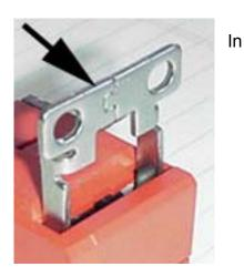
This key is a good example of an item that was designed for manufacture because the irregular 3-D shape is created by simply die-cutting a piece of flat stock, forming it, then punching it to fix it. No machining, welding, or fasteners are required. Material use is efficient.
