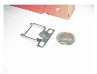
Although it is difficult to see in the photograph, the key is formed from one flat piece of metal. It is stamped out, and then bent. The two ends are brought together and fastened.
