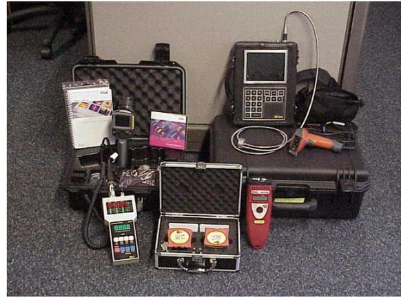
**Figure 9: Toolbox of reliability centered maintenance tools**
