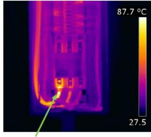
**Figure 5: Image seen through an infrared camera of a hot spot on an electrical panel that may have been missed during a visual inspection**
