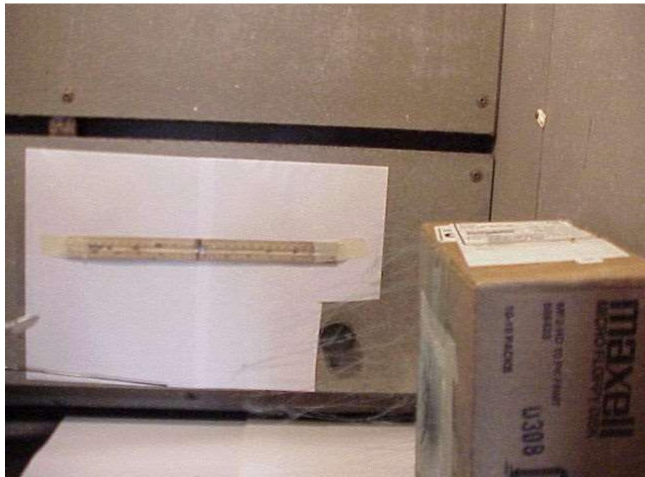
Polystyrene in THF (MW 212,000) – 20kV/ 20cm
