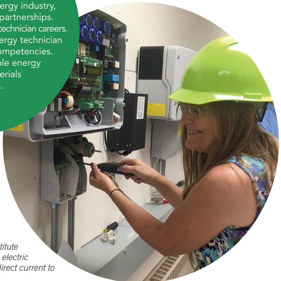
*A CREATE Solar Institute participant wires an electric inverter to change direct current to alternating current.*
