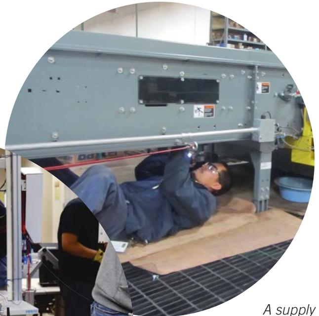
*A supply chain technician repairs a conveyor belt that moves small, light products.*
