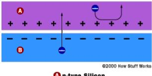
An-type Silicon p-type Silicon The effect of the electric field in a PV cell
