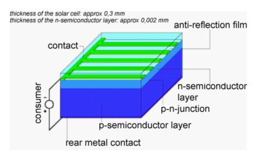
model of a crystalline solar cell<sup>9</sup>
